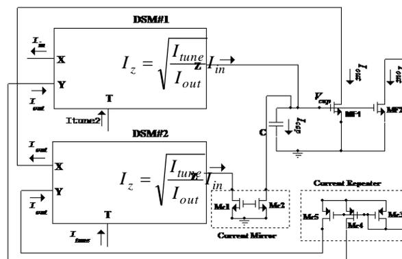
Figure 3: Block diagram of the LPF filter
