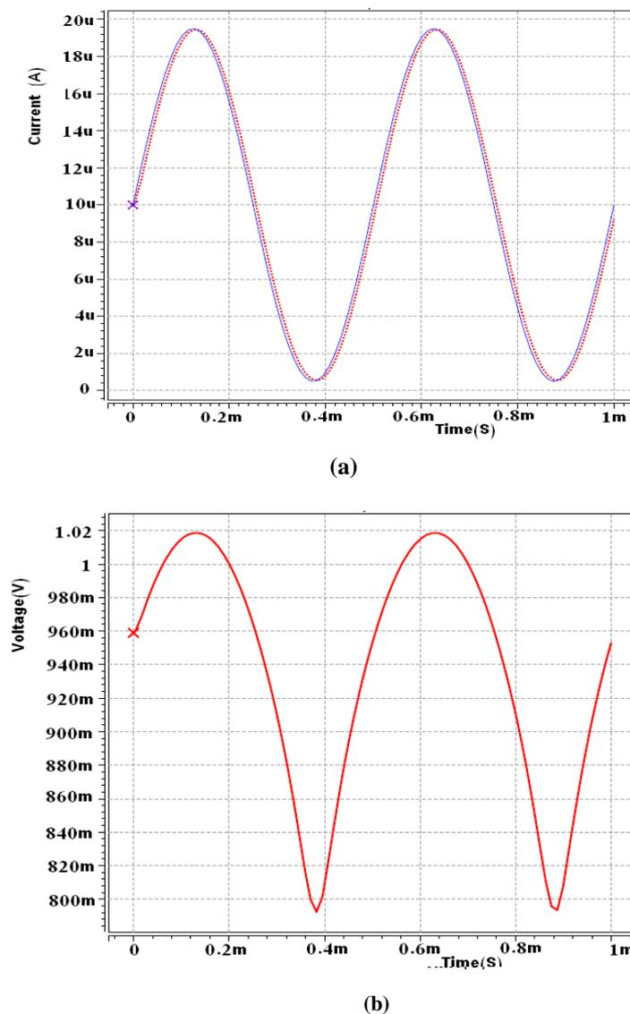
Figure 7: Time response of the LPF; a: Input and output currents, b: Capacitance voltage
