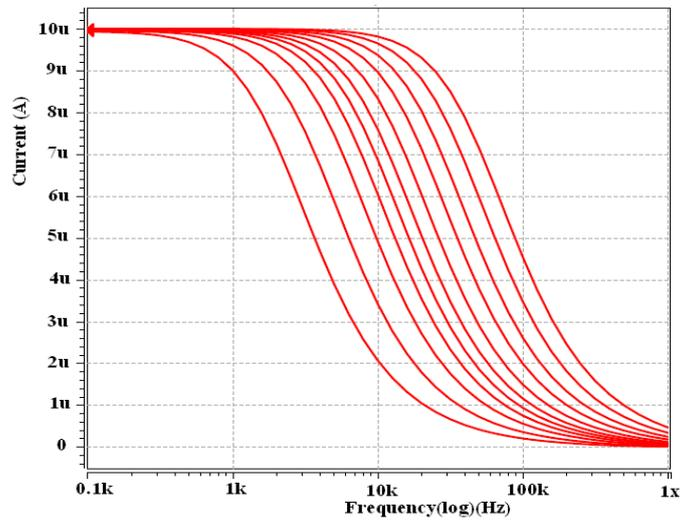
Figure 8: Frequency response of the LPF (for *Itune1* from 0.4uA to 40uA from left to right)
